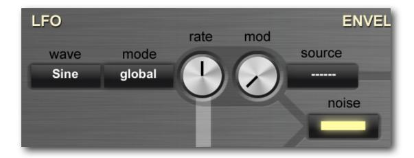
This module provides you with a Low Frequency Oscillator useful for periodic and random sound parameter modulations. The LFO can produce five different modulation waveforms.
