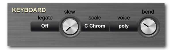
If legato is on, the pitch slides from one note to the next legato played note. The slide parameter controls the time needed to slide between the notes.
