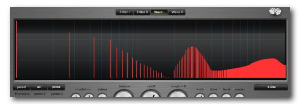
Oscillators provides you with the base material for sound synthesis. They generate periodic oscillations of waveforms with controllable frequency. The spectrum of the six oscillators in Addictive Synth can be freely defined by the amplitude of up to 128 harmonics. You can define two different sets of spectrums labelled I and II with the possibility to morph between them either manual or automatically with the routing possibilities laid out in the control page.
