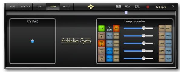
To record a track just tap on the "Rec" button of one of the four tracks. Recording starts with the first key pressed on the keyboard if "play" is not engaged. Recording is always done in "overdub" mode: each recording mixes with already recorded material.
